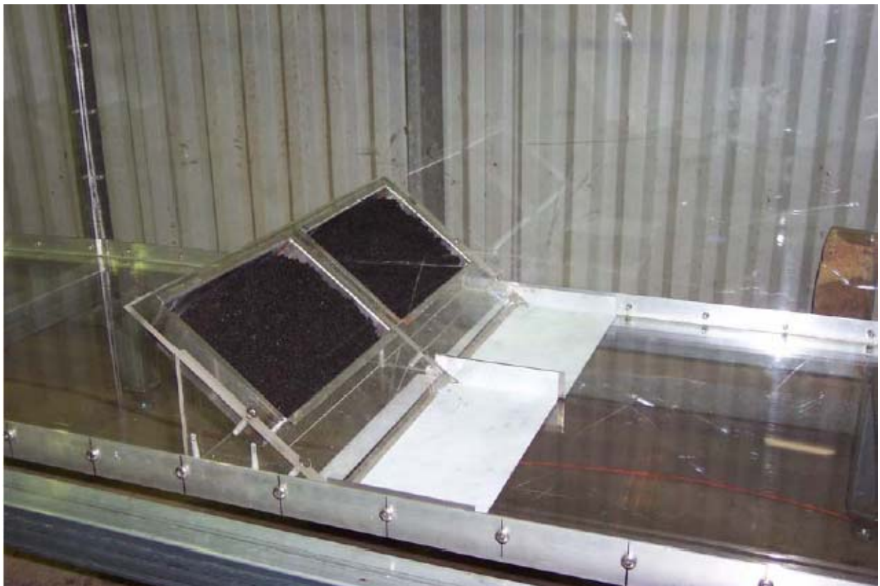
Figure 1: Wind tunnel with two sample trays
