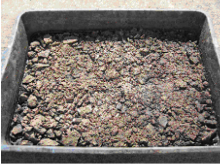
Tray containing road base
